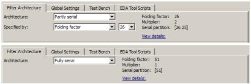
When you click on the **View details** link, the coder displays an HTML report in a separate window. The report displays an exhaustive table of folding factor, multiplier, and serial partition settings for the current filter. You can use the table to help you choose optimal settings for your design.
